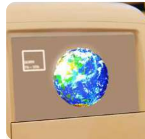
13.5" Transparent Micro LED Panel with World-Leading Resolution
